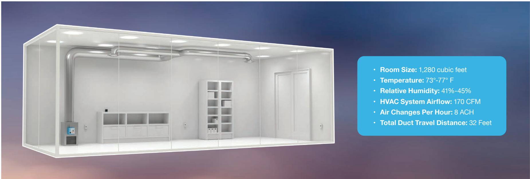
Test conditions represented an active mechanical system and indoor environment through a “Hot Start” scenario where the PuriFi product and HVAC fan system were activated 15 minutes before introducing the pathogen into the environment.
