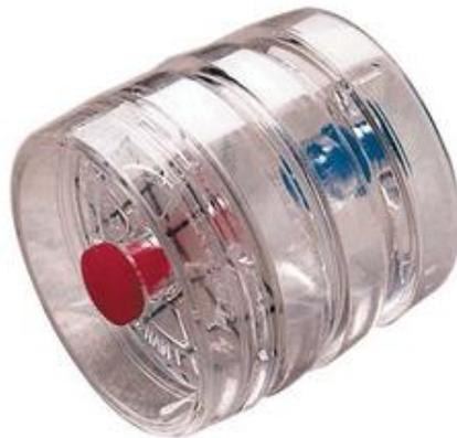
*Figure 2: Sensidyne 37mm directional air flow sample cassette.*
